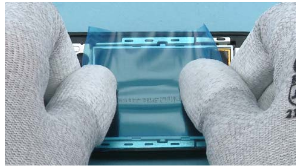
8) Remember to protect the BAFFIN LCD with protective film.
