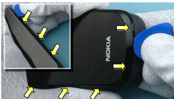
11) Slide the SRT-6 along the phone sides to release all the clips holding the A-COVER.
