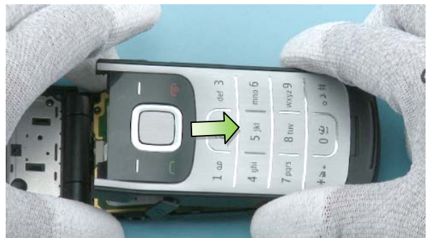
24) Turn the phone and detach the C-COVER in the direction shown.
