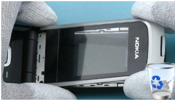
7) Remove the IMD window. The window cannot be used again.
