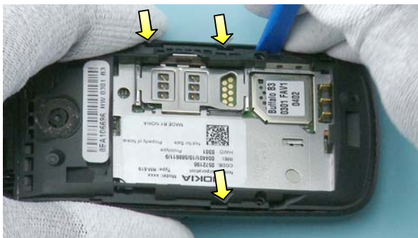
23) Open the phone and release the C-COVER with the SS-93.
